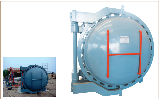
Quick Wedge Lock System Door
